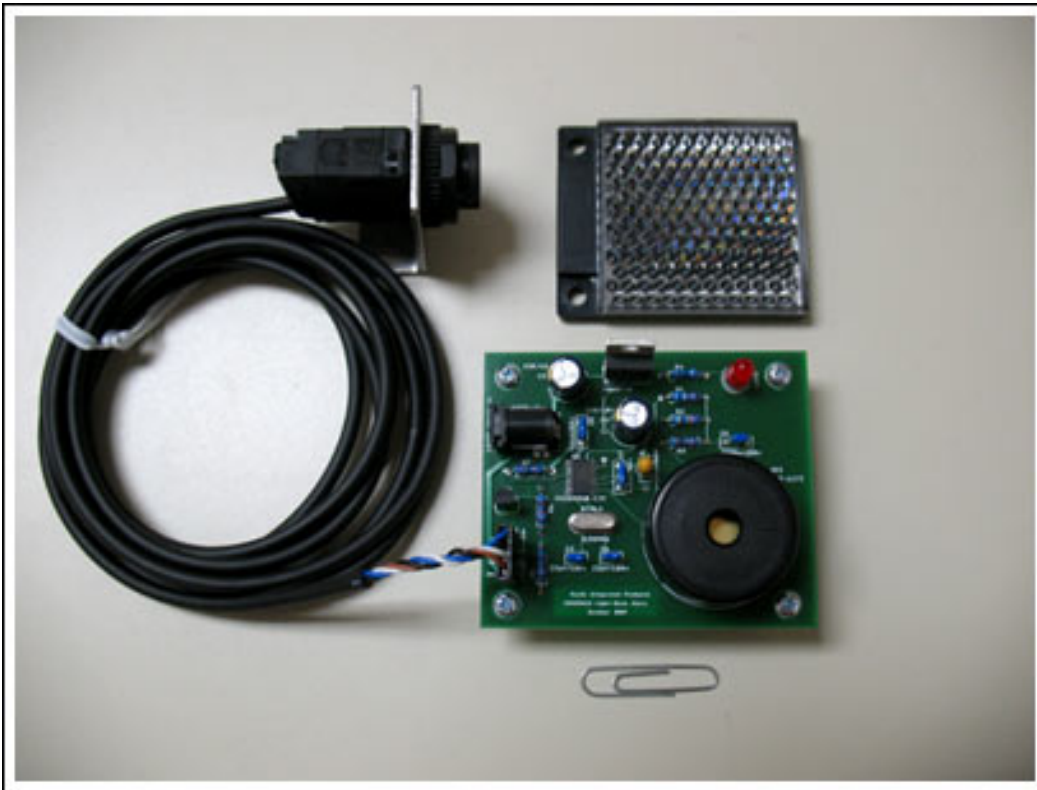
Figure 1. PCB, sensor, and reflector.
