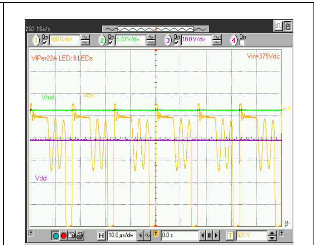
Figure 16. VIPer22A with 8 LEDs at output
