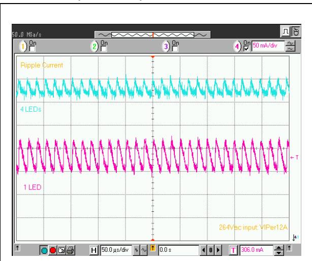
Figure 32. Ripple Current at 264Vac input (VIPer12A)
