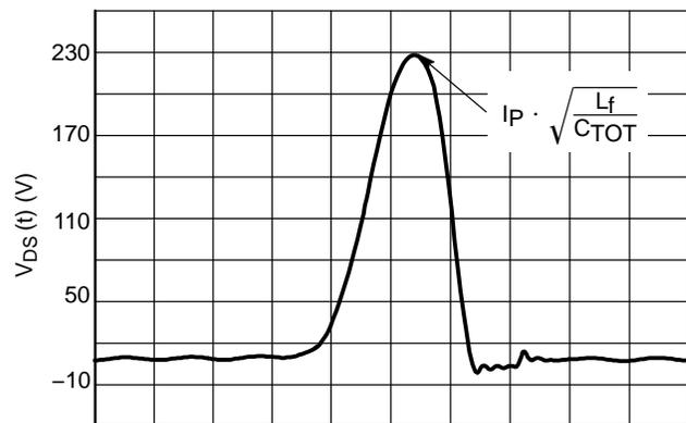
Figure 1. A Truly Resonating  $V_{DS}$  Signal on a Quasi-resonant Flyback Converter
