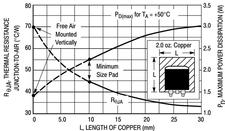
Figure 6. Thermal Resistance vs. Pad Size for a Typical D<sup>2</sup>PAK
