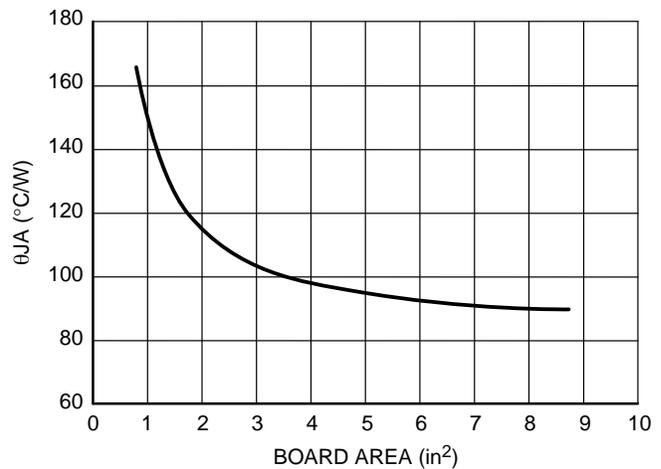
Figure 4.  $\theta_{JA}$  versus Board Area
