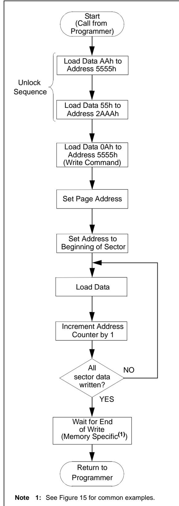
**FIGURE 17: TYPICAL WRITE AND ERASE SEQUENCES FOR “A” AND “B” FLASH FAMILIES**
