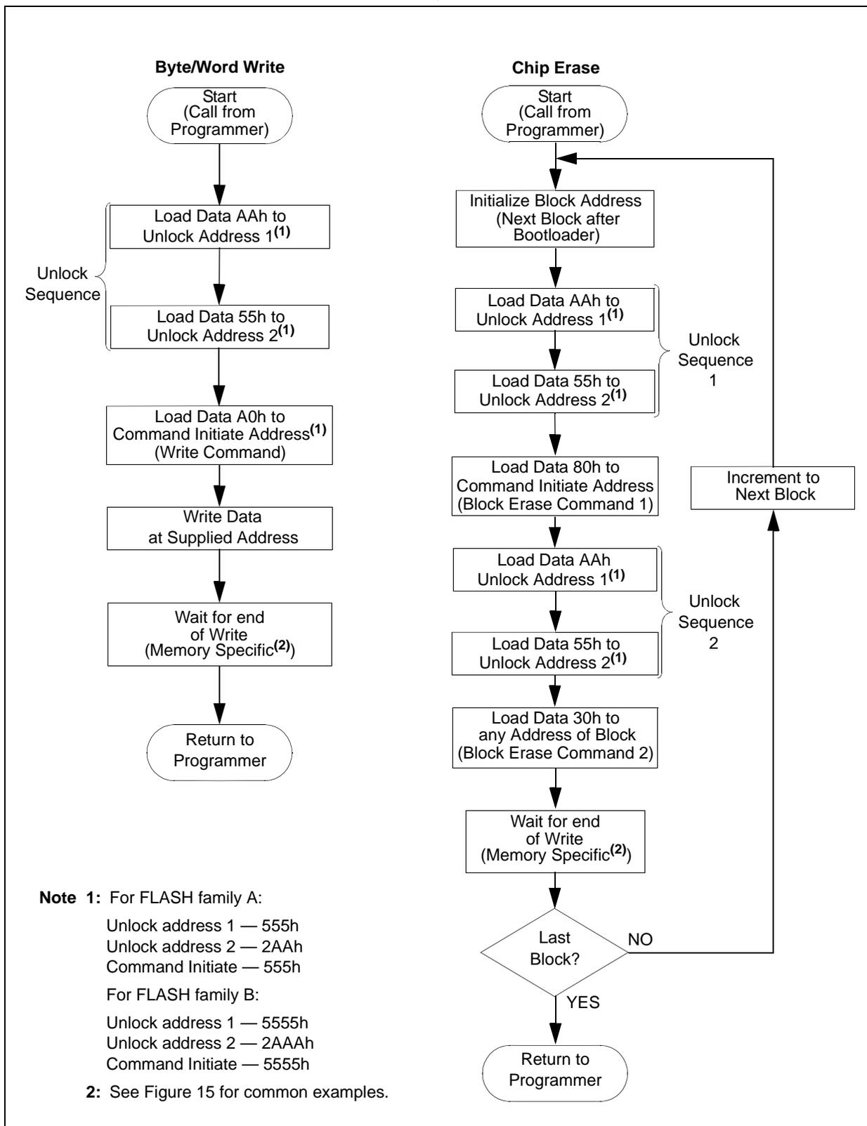
**FIGURE 18: TYPICAL WRITE AND ERASE ROUTINES FOR “C” FAMILY FLASH DEVICES**
