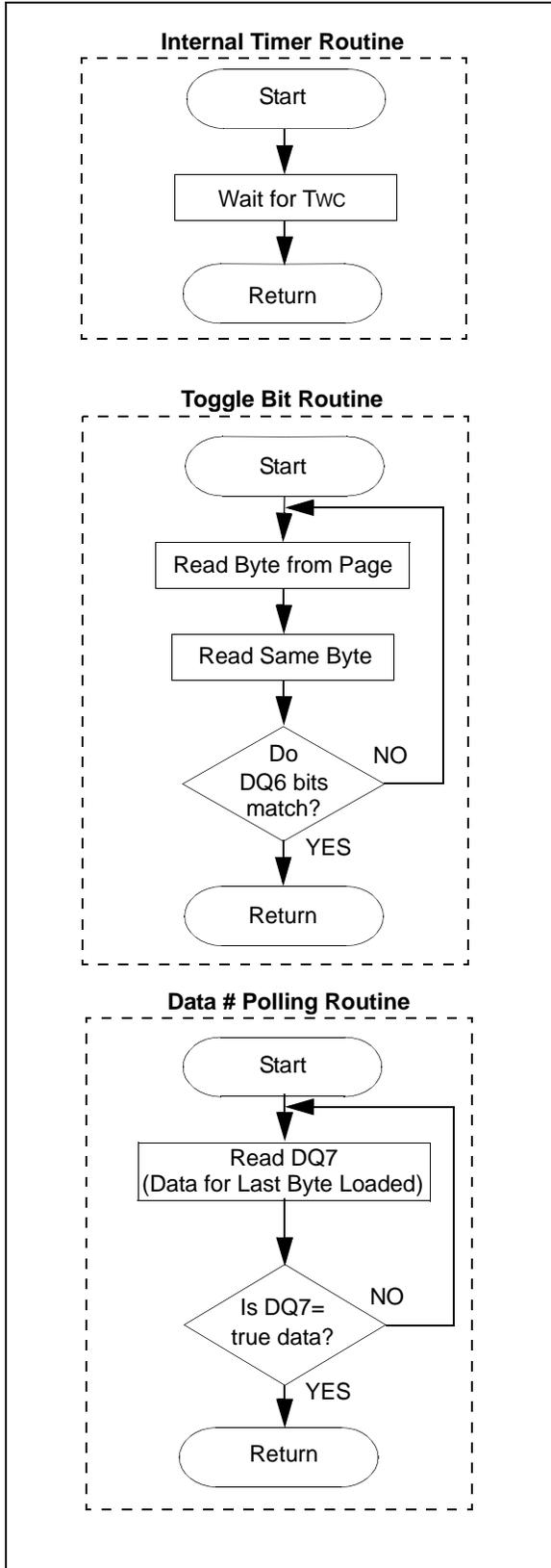
**FIGURE 16: TYPICAL WRITE CYCLE ROUTINE FOR SECTOR-PROGRAM FLASH**
