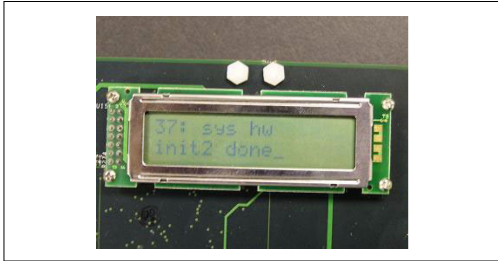
Figure 8. LCD Display for Wind River* VxWorks* Bootloader
