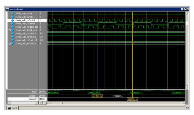
Figure 4 - Post-Route Timing Simulation Results Showing a Data Input Pattern
