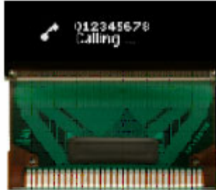
Figure 1-7 · OLED Display Module
