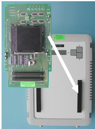
The MB2147-20 Adapter Board has two connectors (ADAPTOR BOARD CONNECTOR A and B) on the backside which fit into the connectors of the Emulator MB2147-01.
