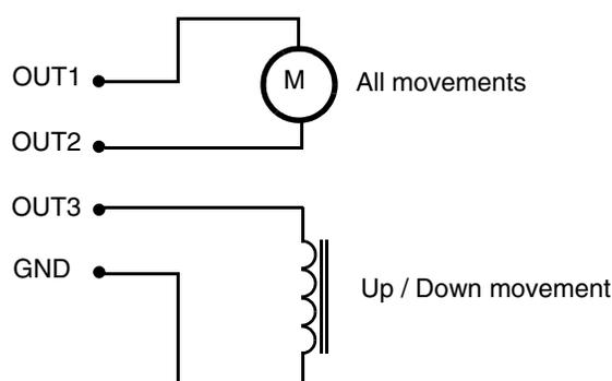
**Figure 9. Electromagnet and Motor Mirror Unit Connection**
