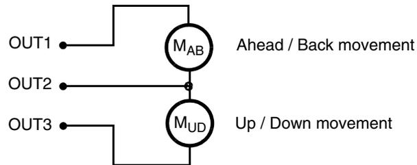
**Figure 8. Two Motor Mirror Unit Connection**
