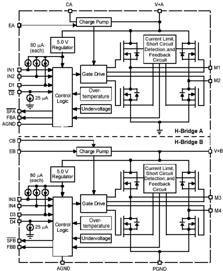
Figure 5. MC33922 (Dual H-bridge) Block Diagram
