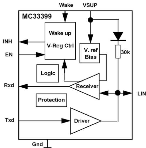
**Figure 4. MC33399 (LIN Physical Interface) Block Diagram**
