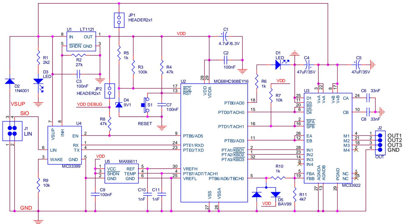
**Figure 6. Slave Unit Schematic Diagram**
